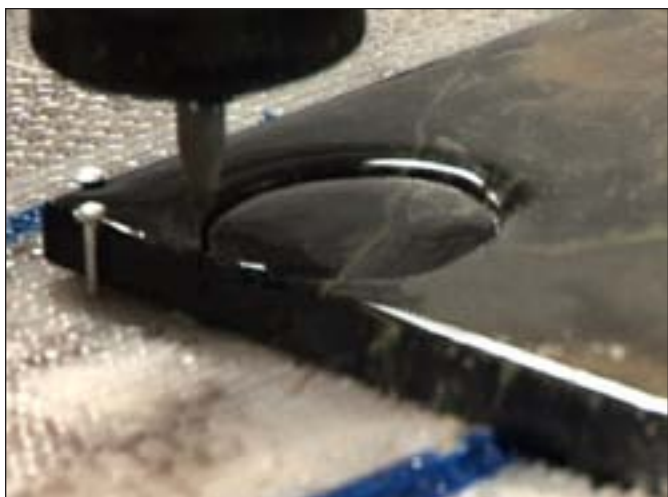
BELOW: RoboCut software controls water jet cutting on this granite countertop.
