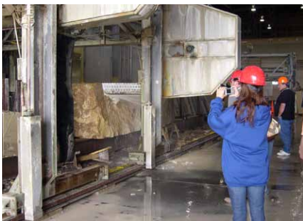
Slab sawing at US Stone Industries’ Herington, KS facility.
