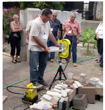
Northern Stone Supply's Greg Osterhout tries out the Mighty C stone splitter at Sturgis Materials stone yard.
