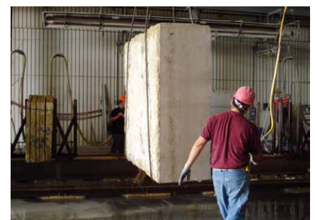
Slab being moved onto saw at Herington facility.
