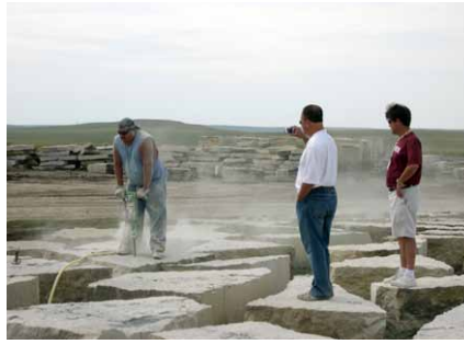
Drilling limestone blocks at US Stone Industries Cottonwood Falls quarry.
