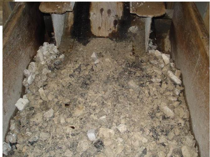
Crushing machine used at Blume's processing facility. Crushed material is currently used as fill for Blume's parking lots.
